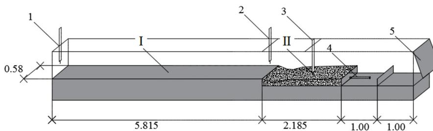
**Figure 4.** Experimental channel scheme (all dimensions in meters). Where: I—solid bottom; II—washout bed (sandy); 1,2—pin water gauge; 3—disc probe; 4—collection chamber; 5—the regulatory gate.
