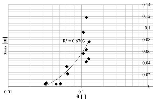
**Figure 11.** Shields parameter and the maximal scour depth correlation graph, where  $\theta$ —dimensionless shear stress in bed region;  $z_{max}$ —maximal scour depth in clear water scour forming process;  $R^2$ —coefficient of determination.
