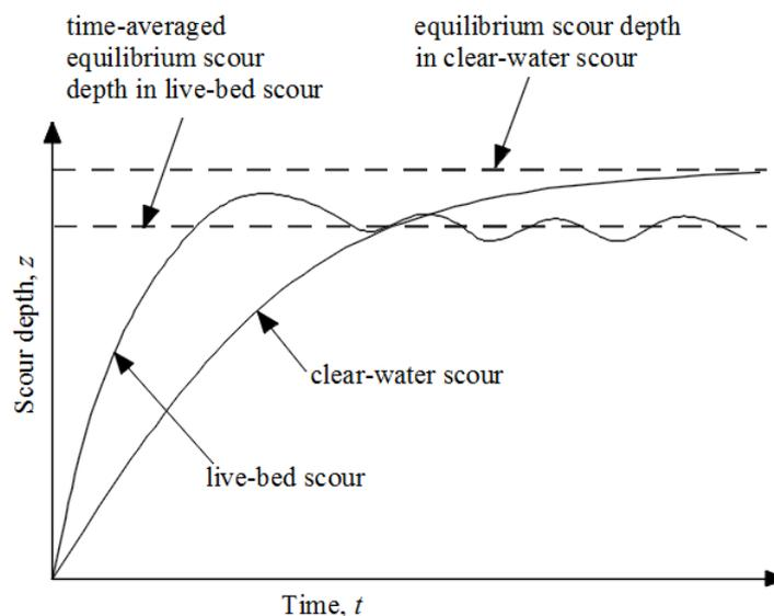
**Figure 1.** Time development of clear-water and live-bed scour [10].
