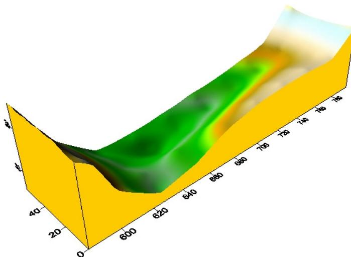
**Figure 6.** Local scour in sandy washout bed (measurement no. 8 in conditions of  $Q_w = 0.040 \text{ m}^3 \cdot \text{s}^{-1}$  and  $H = 0.1 \text{ m}$ ).
