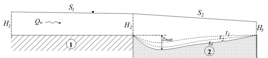
**Figure 2.** Scheme of local scour forming in washable area of sandy bed. Where: 1—solid bottom; 2—sandy washout bed;  $H_1$ ,  $H_2$ ,  $H_3$ —water depth;  $Q_w$ —water flow discharge;  $S_1$ ,  $S_2$ —energy grade line slope;  $z_{max}$ —maximal depth of local scour while achieving stabilization in time  $t_n$  (clear-water equilibrium scour depth);  $t_1$ ,  $t_2$ ,  $t_n$ —shapes of bed while duration of experiment in time.
