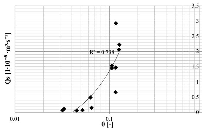
**Figure 10.** Shields parameter and the sediment discharge correlation graph, where  $\theta$ —dimensionless shear stress in bed region;  $Q_s$ —sediment discharge;  $R^2$ —coefficient of determination.
