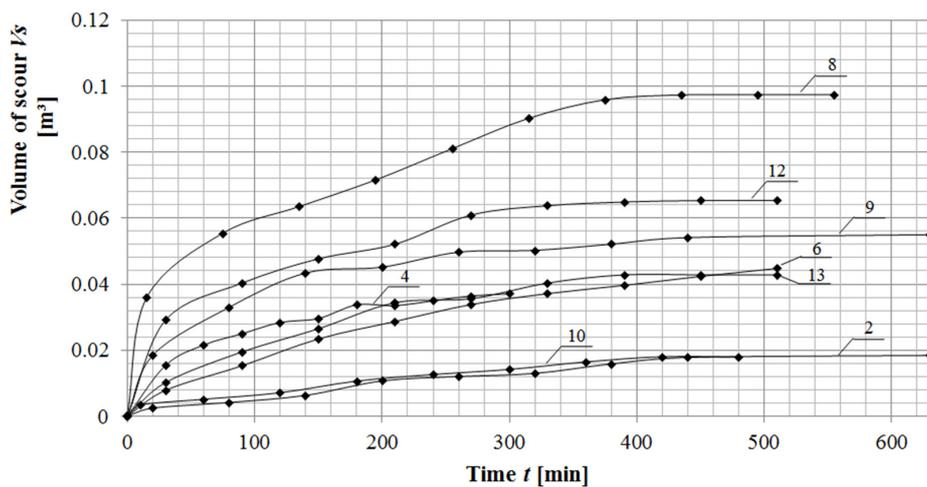
**Figure 8.** Amount of bedload scattered from the dissipation basin (sandy bed) in variants with invisible scour during test runs No 1, 3, 7, 11; Where 1–13 are the numbers of the measurements (compare with Tables 1 and 2).
