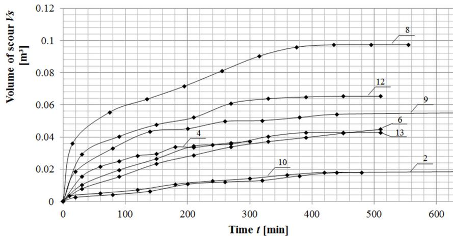
**Figure 7.** Amount of bedload scattered from the dissipation basin (sandy bed) in variants with visible scour during test runs No 2, 6, 8, 9, 10, 12; Where 1–13 are the numbers of the measurements (compare with Tables 1 and 2).
