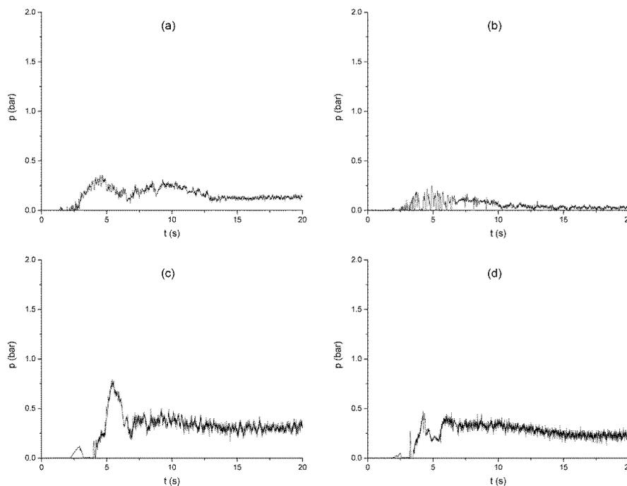
**Figure 4.** Pressure transients for  $\psi_d = 100\%$  with S configuration and: (a)  $\psi_u = 25\%$ ,  $d = 6.4$  mm; (b)  $\psi_u = 25\%$ ,  $d = 25.4$  mm; (c)  $\psi_u = 100\%$ ,  $d = 6.4$  mm; (d)  $\psi_u = 100\%$ ,  $d = 25.4$  mm.
