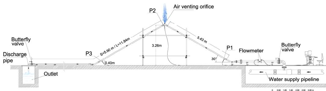
Figure 1. Experimental set-up.
