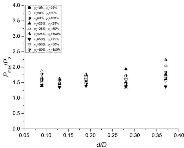
**Figure 9.** Values of  $p_{\max}/p_0$  at varying  $\psi_d, \psi_u, d/D$  (L configuration,  $L_d = 11.84$  m).
