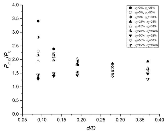
**Figure 8.** Values of  $p_{\max}/p_0$  at varying  $\psi_d, \psi_u, d/D$  (S configuration,  $L_d = 5.90$  m).
