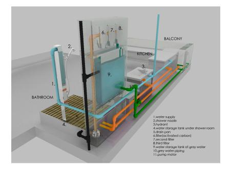
Figure 5. ICGS design introduced to the case.
