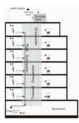
Figure 1. Conventional Greywater System.
