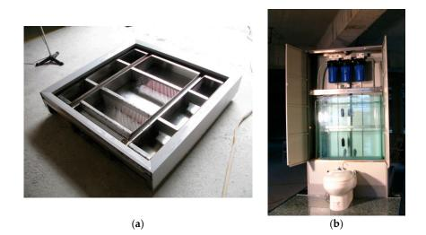
**Figure 3.** Prototype model of greywater processing: (a) Primary filtration and sedimentation; (b) Filtration, sterilization and water storage.
