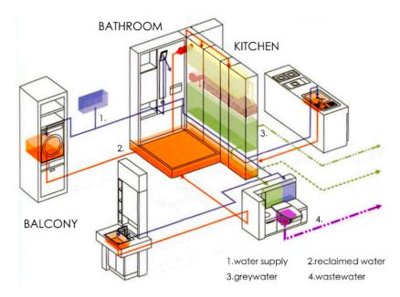
Figure 2. Conceptual diagram of Interior Customized Greywater System (ICGS).
