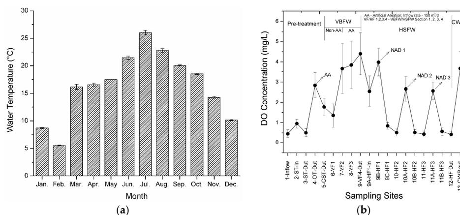
**Figure 2.** The water temperatures and dissolved oxygen (DO) levels in the studied hybrid system. (a) Average monthly water temperatures; (b) Annual average DO concentrations along with the flow routes of the investigated hybrid constructed wetland (CW).
