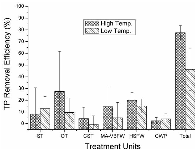
**Figure 4.** Total phosphorus (TP) removal efficiency in different treatment stages during summer and winter.
