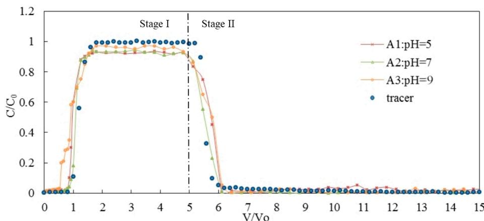
**Figure 3.** Breakthrough curves of silica colloid suspension under different pH values.
