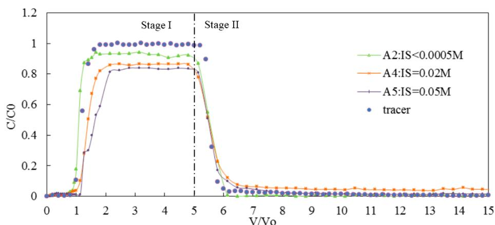
Figure 4. Breakthrough curves of silica colloid under various concentrations of NaCl.
