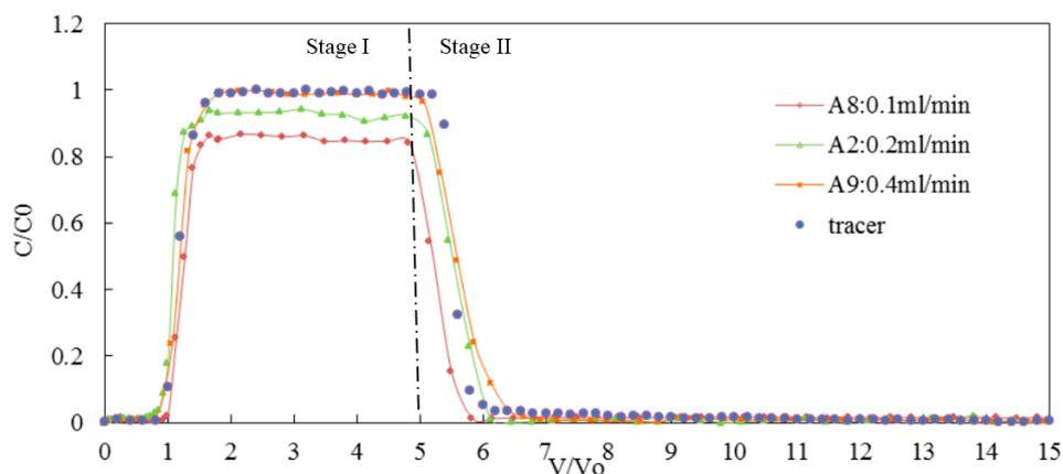
Figure 6. Breakthrough curves of silica colloid under different flow rates.
