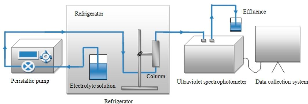
**Figure 2.** Schematic diagram of the experimental setup.
