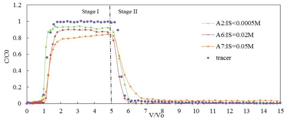
Figure 5. Breakthrough curves of silica colloid suspension under various concentrations of  $\text{CaCl}_2$ .
