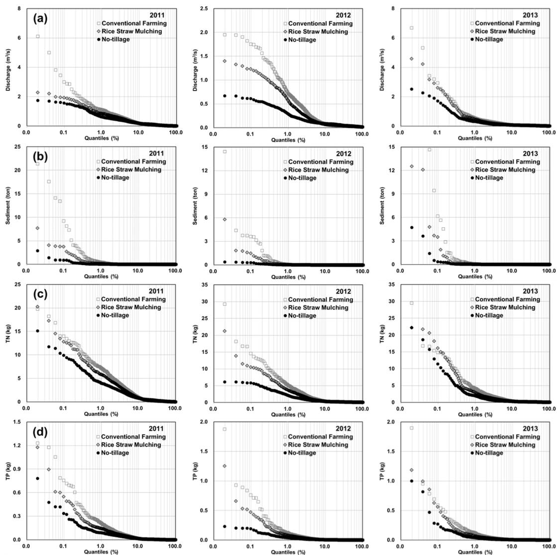
**Figure 6.** Quantile plots of the hourly simulated (a) discharge; (b) sediment; (c) T-N; and (d) T-P for the conventional, rice straw mulching and no-tillage BMP scenarios.
