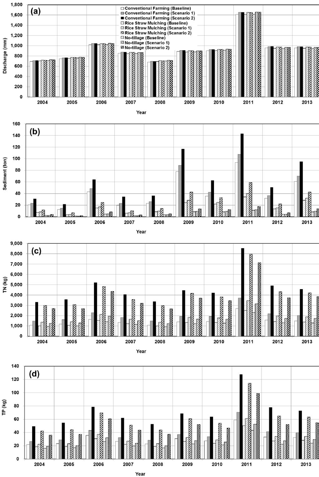
**Figure 8.** Annual change in the hourly simulated (a) discharge; (b) sediment; (c) T-N; and (d) T-P for conventional, rice straw mulching and no-tillage operations when applying change scenarios of upland crop areas
