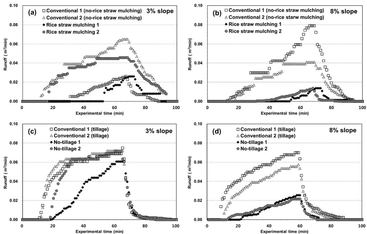
**Figure 5.** Field experiment results for runoff under the (a) rice straw mulching at 3% slope plot; (b) rice straw mulching at 8% slope plot; (c) no-tillage conditions at 3% slope plot; and (d) no-tillage conditions at 8% slope plot.
