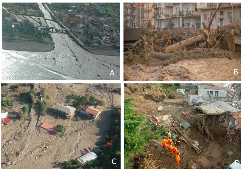
**Figure 1.** (A) The mouth of Longano River on the morning of 23 November 2011, and the bridge collapsed after the flood; (B) tree trunks obstruct the river flow in town center of Barcellona Pozzo di Gotto; (C) debris flows hit Varella village, Mela river catchment; and (D) a debris avalanche struck houses in Scarcelli village, Saponara municipality, and caused three deaths.
