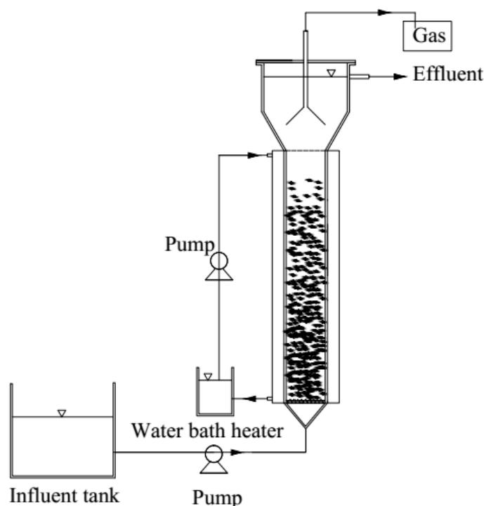
**Figure 1.** Schematic diagram of the Anammox-up-flow anaerobic sludge blanket (UASB) reactor.
