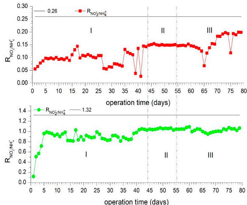
**Figure 3.** Ratios of nitrite consumption to ammonium consumption ( $R_{NO_3^-/NH_4^+}$ ) and nitrate production to ammonium consumption ( $R_{NO_2^-/NH_4^+}$ ) during the Anammox process.
