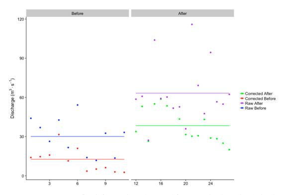
**Figure 7.** Average winter flow before regulation (year 1–10) for corrected and raw data (red and blue, respectively) and after regulation (year 12–26) for corrected and raw data (green and purple, respectively). The whole lines show the mean of each category of data.
