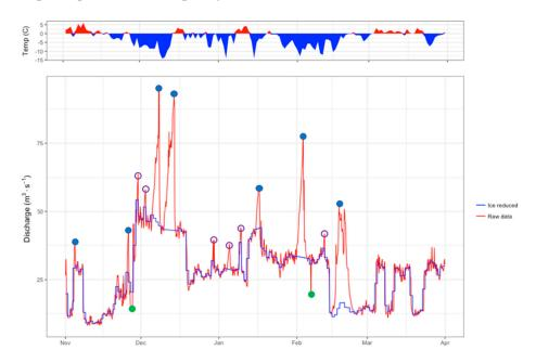
**Figure 2.** Air temperature (top panel) and identified peaks for one year at Syrstad (lower panel). Open circles are peaks that are considered natural, closed blue circles high peaks due to ice, and closed green circles are low peaks. Note that the variability of flow is driven by hydropower releases.
