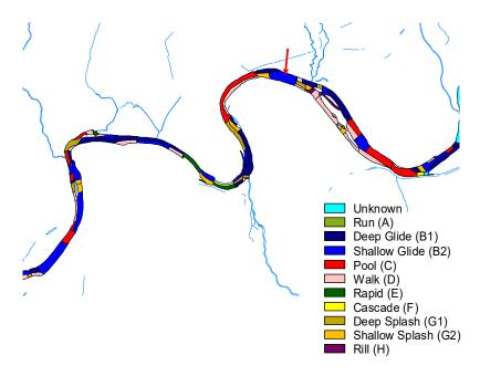
**Figure 8.** A section of the Orkla river mapped by the classification system described by [39]. The arrow indicates the position of the Syrstad gauge located in a shallow glide, which shows frazil ice accumulation over winter.
