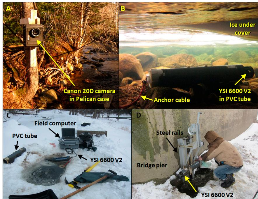
**Figure 2.** (A) Automated Canon 20D digital camera in adapted pelican case at Site M2; (B) aquatic view of the YSI 6600 V2 in its PVC tube at Site M3; (C) retrieving and downloading the YSI 6600 V2 at Site E4 in February 2012; and (D) retrieving and downloading the YSI 6600 V2 prior to breakup at Site E3.
