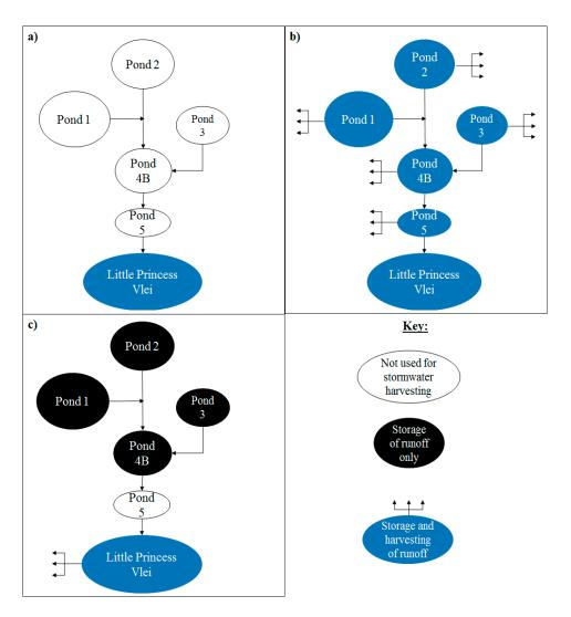
Figure 4. Schematic of RTC options: (a) RTC Strategy A; (b) RTC Strategy B; (c) RTC Strategy C.
