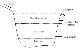
Figure 2. Conceptual design of an open storage stormwater harvesting system (After Mitchell et al. [5]).
