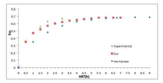
Figure 5. Effect of HRT on SS Efficiency.
