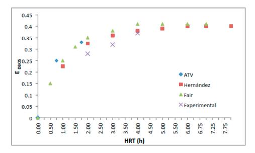
**Figure 6.** Effect of HRT on BOD<sub>5</sub> Efficiency.
