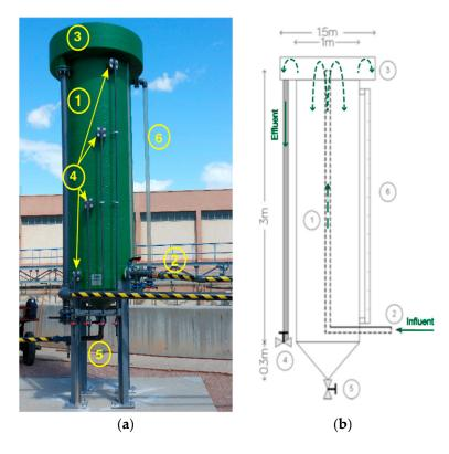
Figure 2. Semi-technical PST: (a) picture; (b) schematic diagram.
