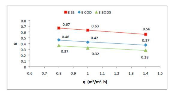
Figure 3. Effect of q on SS, COD and BOD<sub>5</sub> Efficiency.
