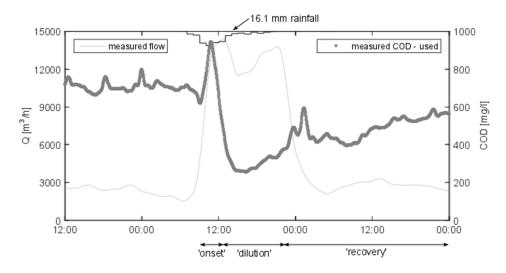
**Figure 3.** Wet weather flow (WWF) dynamics during the stages of a storm event on 12 June 2008 in Eindhoven Stad catchment.
