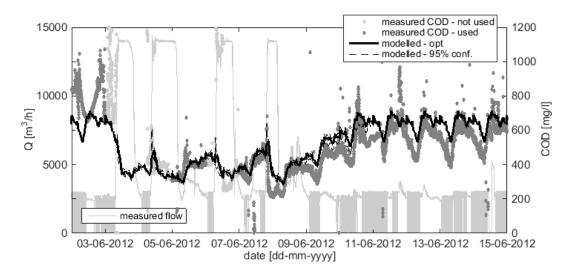
**Figure 10.** Model vs. monitoring data: COD<sub>total</sub> in the WWTP influent for Eindhoven Stad. The small peaks in influent concentration (typically referred to as 'first flush') at the beginning of storm events on 4 June, 6 June and 8 June are adequately represented by the model.
