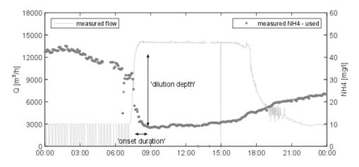
**Figure 5.** Parameters of parabolic function that describes the delayed dilution of the quality parameters compared to the flow.
