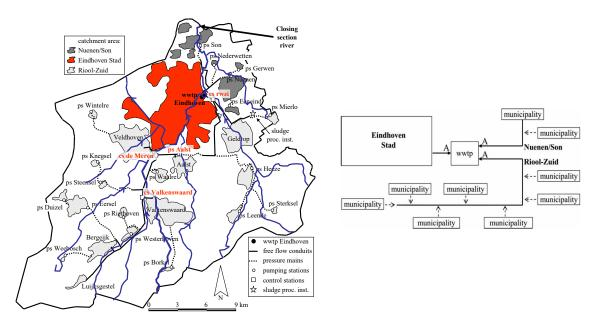
**Figure 1.** Wastewater system of Eindhoven (**Left**) and its receiving streams and schematic lay out of the wastewater system; (**Right**) Figure reproduced with permission from [23].
