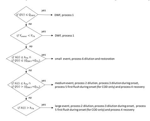
**Figure 4.** Selection of water quality processes to be superimposed on process 1 during dry weather (DWF), using information on hydraulics. The abbreviation Th in the figure is short for threshold.
