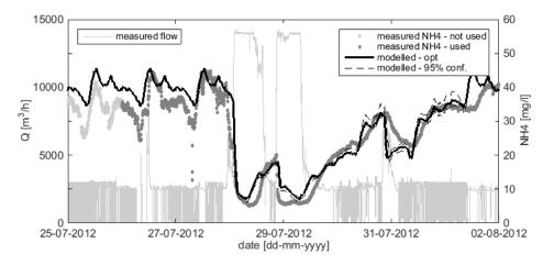
**Figure 8.** Model vs. monitoring data: NH<sub>4</sub> concentration in the wastewater treatment plant (WWTP) influent.
