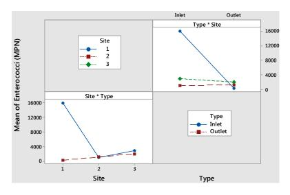
**Figure 1.** Interaction plots for enterococci for three bioretention cells in Grove, Oklahoma (Site 1 = GLA: Grand Lake Association, Site 2 = GHS: Grove High School, Site 3 = ECP: Elm Creek Plaza, Type = Inlet and Outlet, Inlet = inflow from the inlet, Outlet = outflow from the underdrain).
