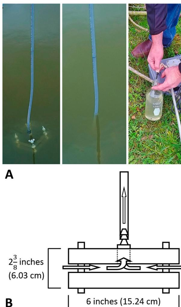
**Figure 3.** Use and action of the water sampler. (A) Lowering the sampler into the water by its tubing and subsequent sample collection in a rinsed and sterilized bottle. (B) Schematic diagram showing the mechanism of water sample collection (arrows indicate water flow). A major advantage of this design is that the water sample is pulled between the two acrylic squares within a space of 1 cm, allowing for high-resolution sampling and precise data collection.
