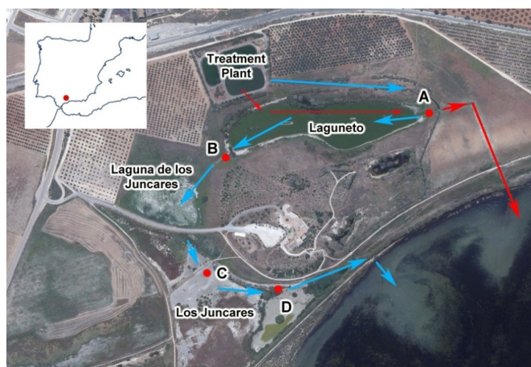
Figure 1. Location map of the study area, sampling points, and water flow through the semi-natural ponds system (blue arrows) direct to the Ramsar wetland. Before restoration in 1996, water flows followed the red arrows, but this is no longer possible.
