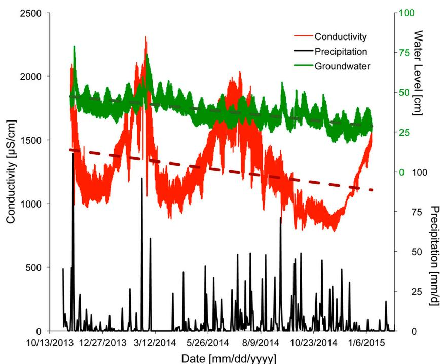
**Figure 9.** Time series plot showing variations in rainfall (black), groundwater level (green), and conductivity of water (red) in well R3 observed between November 2013 and February 2015. Linear fits to the data are denoted by dotted lines.
