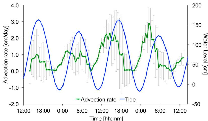
**Figure 6.** Time series showing ocean water levels (tides, in blue) and the computed submarine groundwater discharge (SGD, in green) advection rates. The error bars denote  $\pm 1$  standard deviation.
