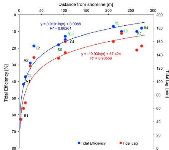
**Figure 4.** Tidal efficiency and tidal lag calculations for groundwater wells. Groundwater well locations shown in Figure 1. Data for groundwater wells R1–R11 (green) were published by Gingerich, 1992 and normalized to 3 m depth using a linear relationship.
