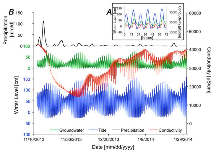
**Figure 5.** Time series plots showing tidal forcing of groundwater levels and salinity (Well C1), as well as the observed response to a large rain event. (A) From 11 November 2013 through 29 January 2014. (B) From 1 December through 4 December 2013. Precipitation gauge data available from NASA/RTS (2017) [46].
