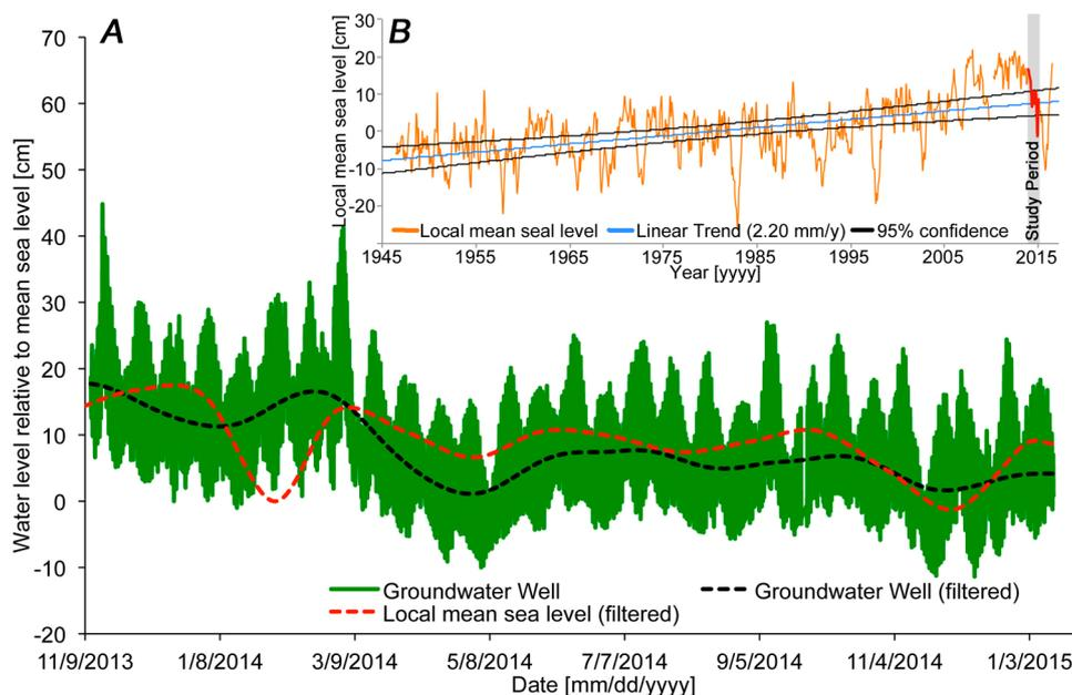
**Figure 10.** Time series of sea-level forcing and well response; (A) Comparison of groundwater levels and sea levels during the study at Well R11; (B) Local mean sea-level curve from 1945 to 2017. Period pertaining to this study is marked in gray. Sea level data for Kwajalein Atoll from NOAA [52]. A Butterworth filter with a frequency cutoff of 60 d was used to filter data.
