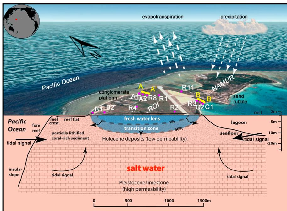
**Figure 1.** Satellite image and conceptual drawing of the shallow aquifer system of Roi-Namur, Kwajalein Atoll, Marshall Islands. Location of shallow groundwater monitoring wells (magenta dots) and time-series electrical resistivity transects (yellow lines) are indicated.
