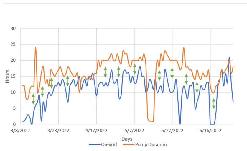
**Figure 9.** On-grid electricity supply and running time of water pumps in hours per day. Green arrows signify the energy gap covered by renewable energy due to national grid outages. *Source: Authors.*
