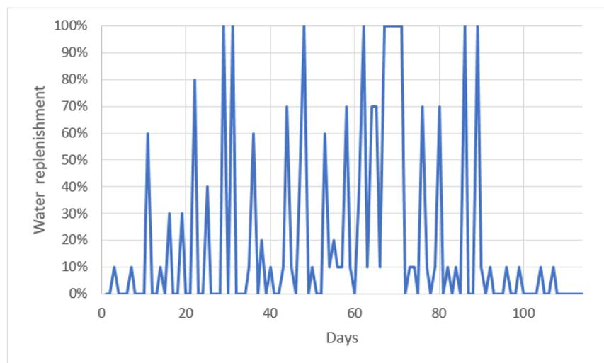
**Figure 8.** The filtration cleaning and water replenishment in the SANFU II RAS in one cycle. *Notes: Filtration cleaning always took place when the water replenishment was above 5 percent. Source: Authors.*
