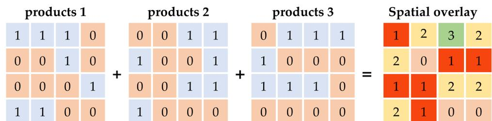
**Figure 3.** The map of the spatial overlay of the different land cover products. **Legend:** Land cover type: 1—forest; 0—non-forest; Overlay results: 0—background; 1—completely inconsistent; 2—basically consistent; 3—completely consistent.
