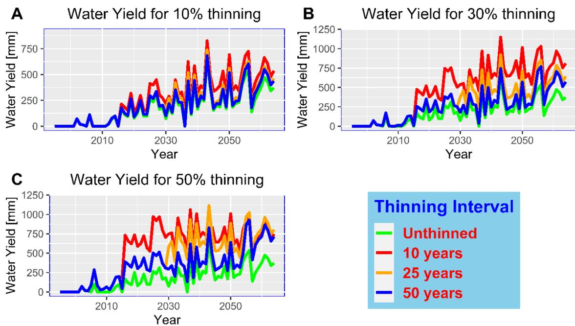
**Figure 4.** Water Yield for (A): 10%, (B): 30%, and (C): 50% thinning in different thinning intervals.
