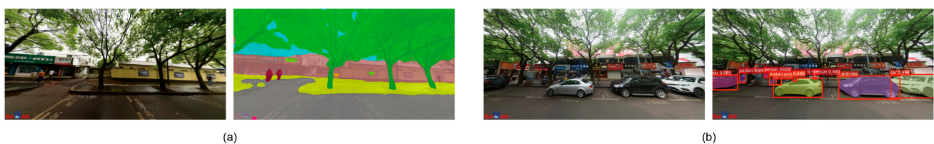
Figure 4. Examples of CV segmentation results. (a) DeeplabV3 semantic segmentation. (b) Mask R-CNN instance segmentation.
