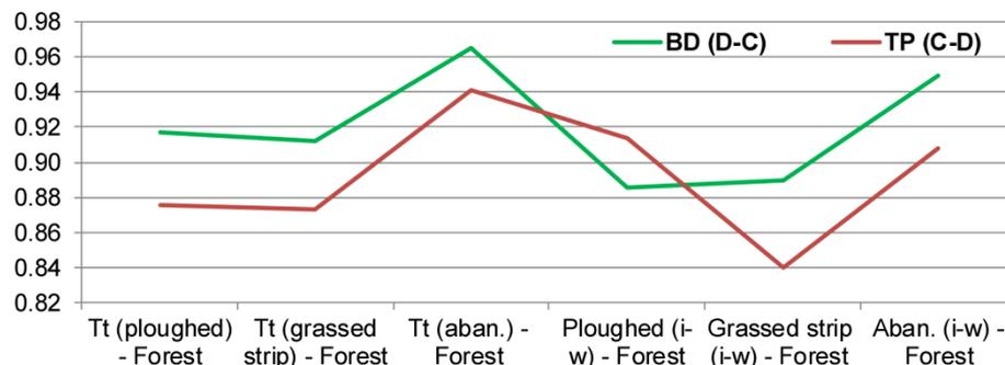
**Figure 6.** Resilience for BD and TP (Tt, tractor track; i-w, space between the wheels; BD, bulk density; TP, total porosity; D, disturbed soil; C, control soil).
