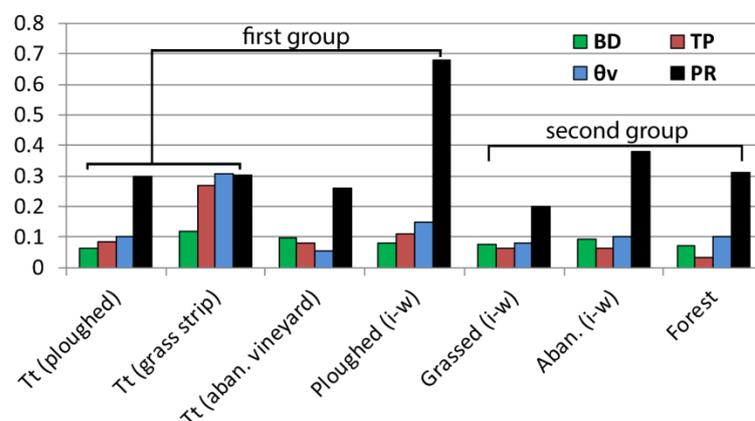
**Figure 4.** Entropy for soil properties (Tt, tractor track; i-w, space between the wheels; BD, bulk density; TP, total porosity;  $\theta_v$ , volumetric moisture; PR, penetration resistance).
