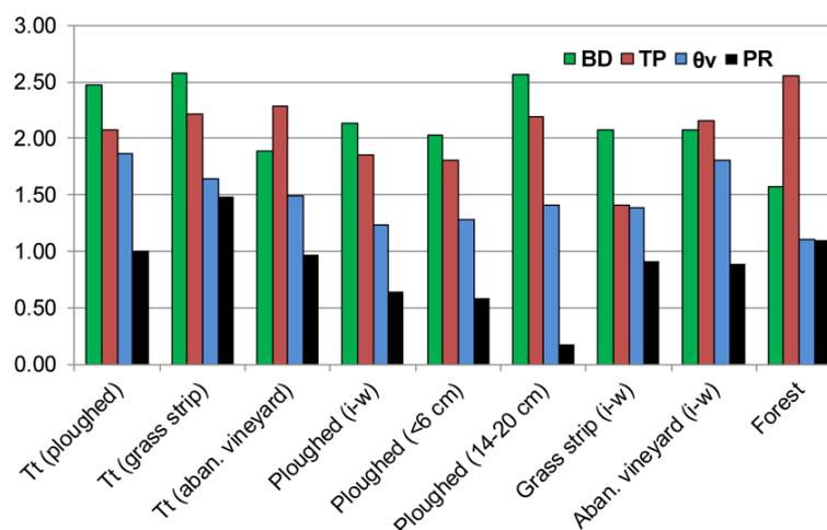
**Figure 5.** Interquartile report index for soil properties (Tt, tractor track; i-w, space between the wheels; BD, bulk density; TP, total porosity;  $\theta_v$ , volumetric moisture; PR, penetration resistance).
