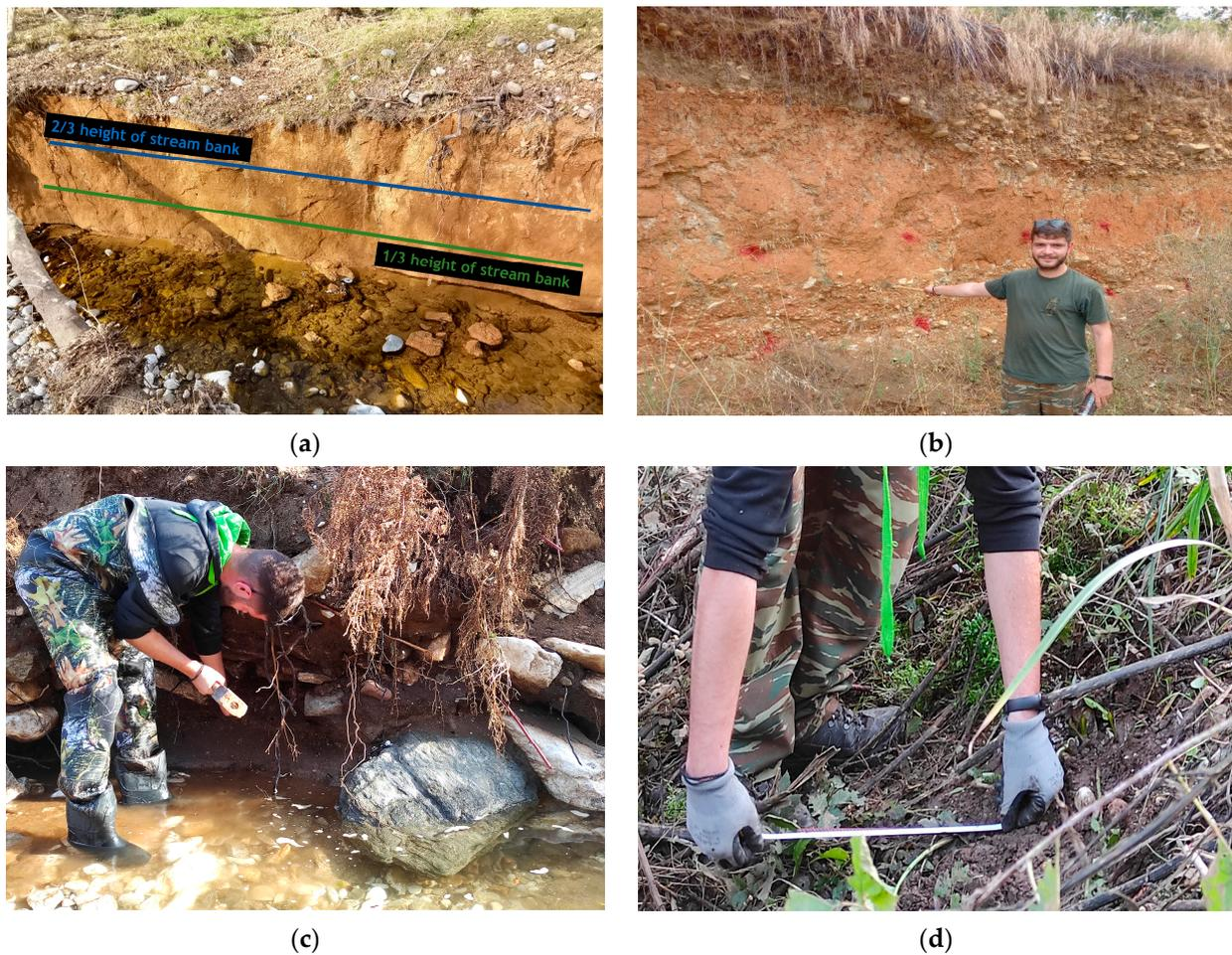
**Figure 3.** Examples of stream bank erosion pins in Kallifytos torrent: (a) the two different height zones of erosion pin placements; (b) erosion pins marked with red paint for better identification; (c) placement of the erosion pins; (d) measuring erosion/deposition of the erosion pins.
