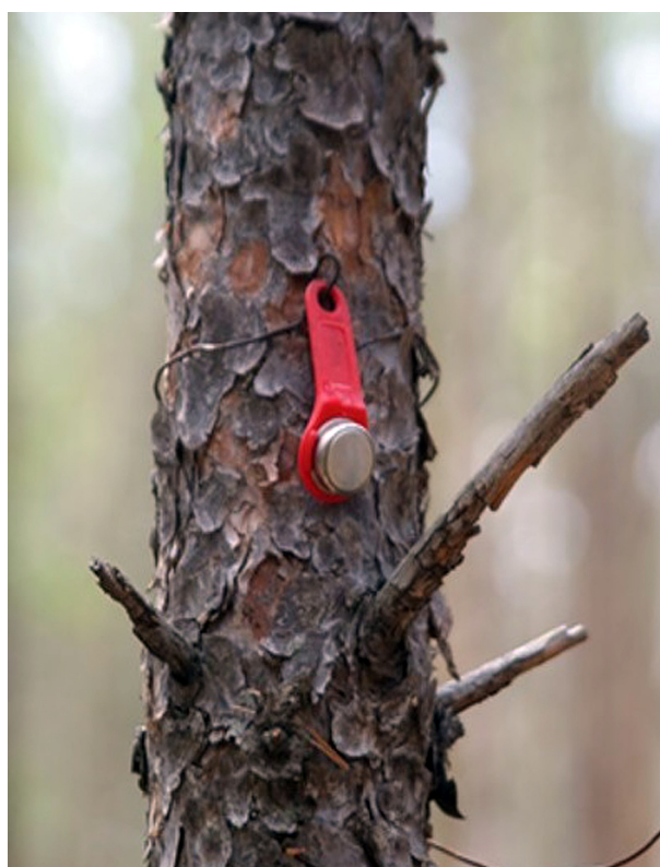
Figure S14. Thermochrone device mounted at north side of a pine tree at 2 m above surface for air temperature in-situ monitoring.
