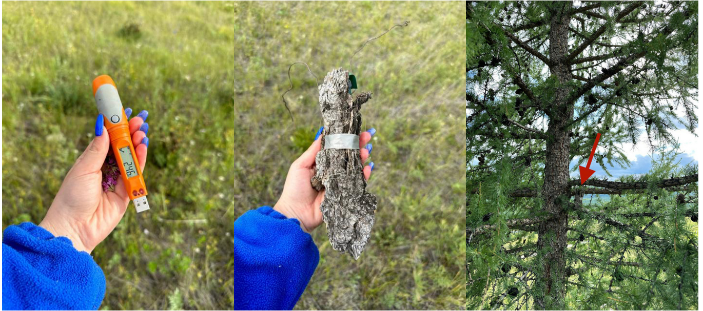
Figure S15. Elitech RC-51H temperature data logger used for air temperature monitoring (left), device covered by larch bark for hidden installation (center), device mounted at north side of a pine tree at 2 m above surface for air temperature in-situ monitoring (right).
