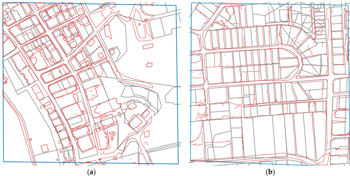
Figure 10. Overlay of workflow results and reference cadastral maps: (a) and (b) illustrate region 1 and 2 respectively.
