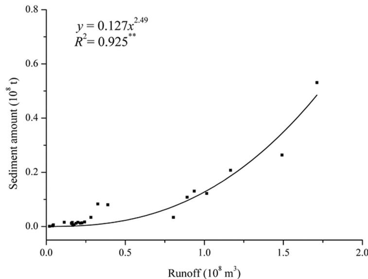
**Figure 6.** The relationship between runoff and sediment.  $x$  is the runoff and  $y$  is the sediment amount.  $R^2$  is the correlation coefficient. \*\* means the correlation was significant at the 0.01 level.
