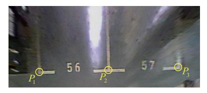
**Figure 13.**  $P_1P_2$  and  $P_2P_3$  are two entrance-line candidates for two perpendicular parking-slots while  $P_1P_3$  is an entrance-line candidate for a parallel parking-slot. Actually,  $P_1P_3$  is invalid and should be removed.
