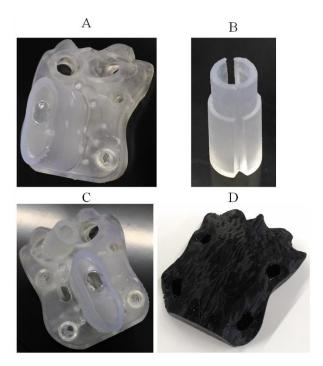
**Figure 8.** The template (**A**) and the left guide (**B**) generated by stereolithography; the template with the left guide inserted (**C**); the support, generated by Fused Filament Fabrication (FFF), reproducing the surface of the sacrum (**D**).
