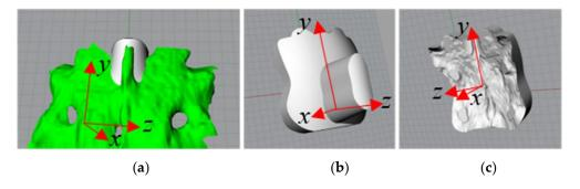
**Figure 6.** (a) Loft surfaces filling blank areas; the model of the template, (b) top view; (c) bottom view; x–y is the sagittal plane, y–z is the coronal plane and z–x is the transverse plane.
