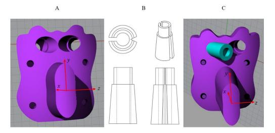
**Figure 7.** Template with tapered drilling (**A**); standard projections views of the guide with the notch and an incomplete section (**B**); final template with the left guide and upper holes (**C**); x–y is the sagittal plane, y–z is the coronal plane and z–x is the transverse plane.
