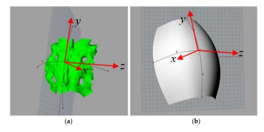
**Figure 4.** Curves (**a**) defining the upper surface (**b**) of the template; x–y is the sagittal plane, y–z is the coronal plane and z–x is the transverse plane.
