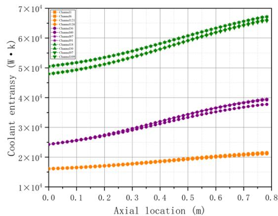
Figure 7. Distribution of coolant entransy in flow process.
