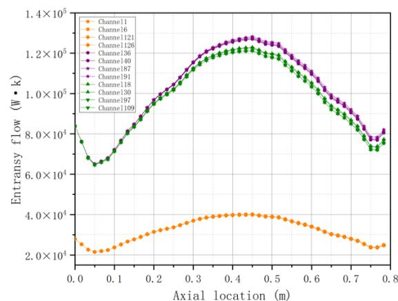
Figure 8. Distribution of entransy flow in heat transfer process.
