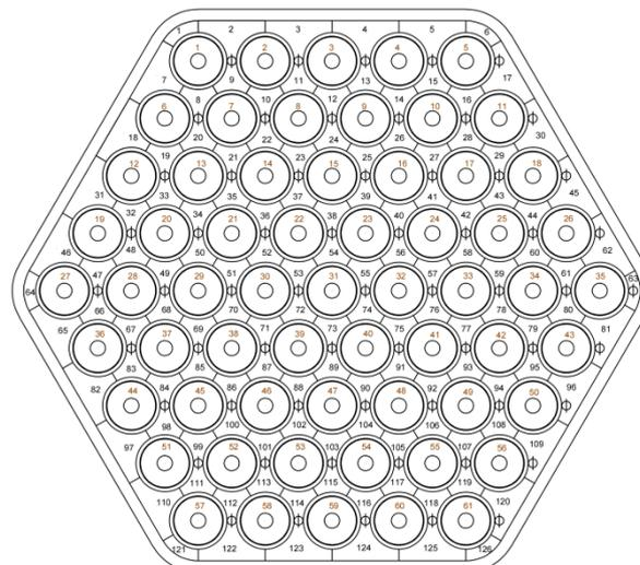
**Figure 1.** Subchannel division of fuel assembly.
