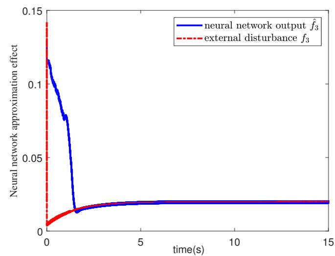
Figure 14. Neural network approximation results of the external disturbance  $f_3(t_k)$ .
