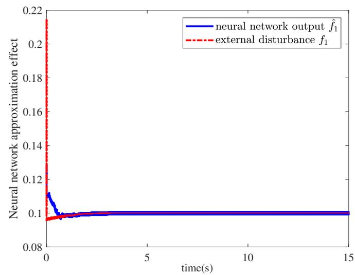
Figure 12. Neural network approximation results of the external disturbance  $f_1(t_k)$ .
