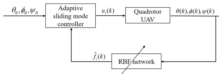
Figure 2. Diagram of the RBF neural-network-based adaptive sliding-mode control algorithm.
