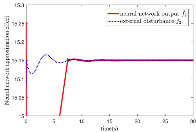
**Figure 7.** Neural network approximation results of the external disturbance  $f_2(t_k)$ .
