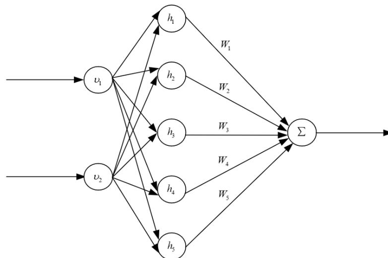
Figure 1. RBF neural network structure diagram.
