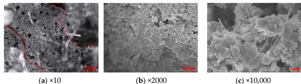
Figure 13. SEM image of the bonding interface.
