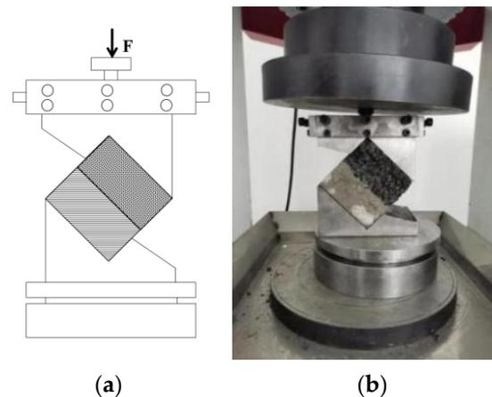
**Figure 3.** Composite specimen interfacial oblique shear test: (a) design drawing; (b) real-shot picture.
