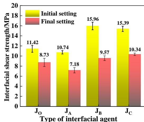
Figure 8. Surface shear strengths of the composite specimens.
