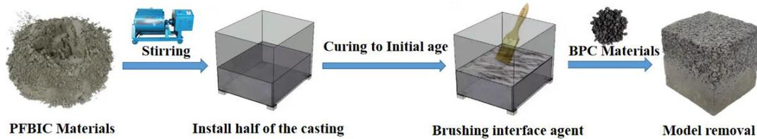
**Figure 2.** Specimen forming process.
