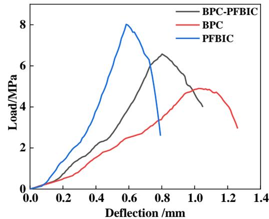
Figure 11. Three-point bending load–deflection curves.
