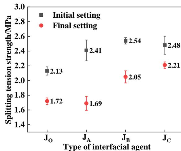
Figure 9. Splitting tensile strengths of composite specimens.
