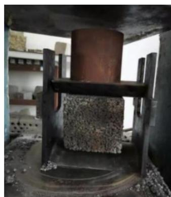
**Figure 4.** Composite specimen splitting tensile test.
