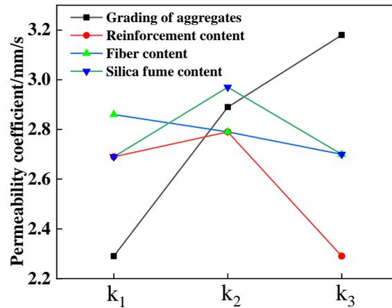
Figure 7. Permeability coefficient change trend.
