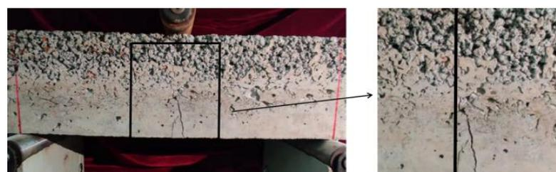
Figure 12. Three-point flexural experiment after fracture existence conditions and a cross-section of the specimens.
