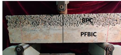
**Figure 5.** Three-point bending test specimens and experimental method.
