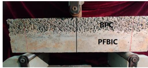
**Figure 5.** Three-point bending test specimens and experimental method.
