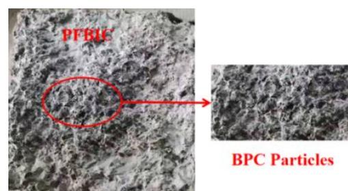
Figure 10. J<sub>B</sub> interface agent composite specimen after the splitting failure interface condition.
