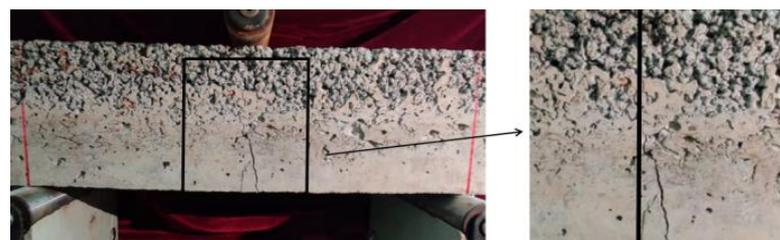
Figure 12. Three-point flexural experiment after fracture existence conditions and a cross-section of the specimens.
