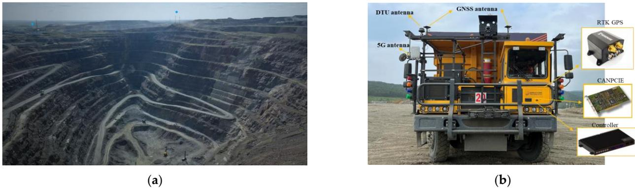
**Figure 8.** Experiment environment. (a) The actual environment of mining site at Bayan Obo. (b) The autonomous truck equipped with 5G antenna, RTK-GPS.
