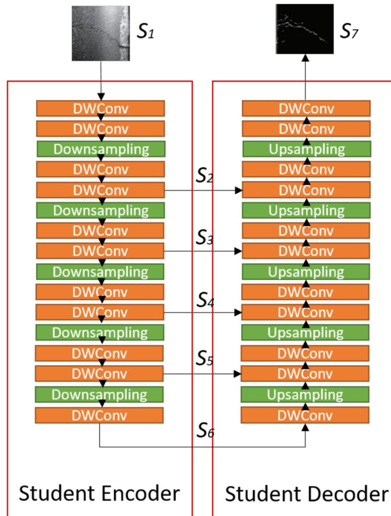
Figure 3. The ultra-light-weighted model (ULNet).
