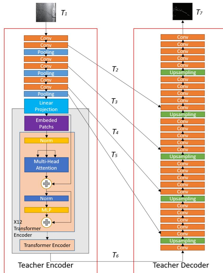
**Figure 2.** The Transformer-based UNet (TBUNet).
