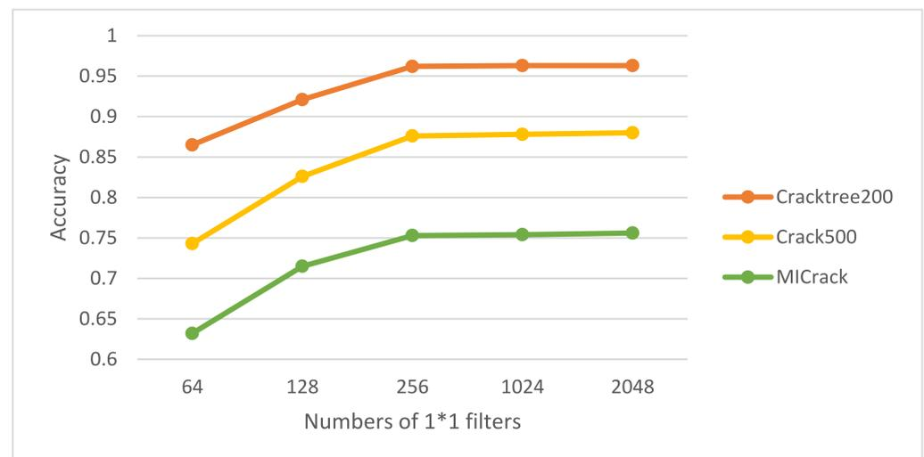
**Figure 6.** Effects of using different numbers of  $1 * 1$  filters in DWConv in ULNet.
