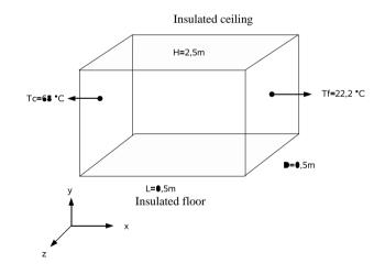
The code used for the simulation is based on a finite difference scheme, explicit in time [29]. The time step is  $2 \times 10^{-4}s$  and the grid size  $(62 \times 62 \times 18)$ . We use the experimental results in [30] as reference solution.
