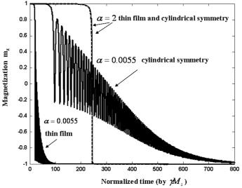
The symmetric effects on magnetization switching behavior for different damping parameters can be understood through analysis of the LLG equation at zero temperature. Without thermal fluctuation and spin torque terms, the LLG in spherical coordinates is:
