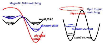
Solid line: Energy level Dash line: magnetization motion
