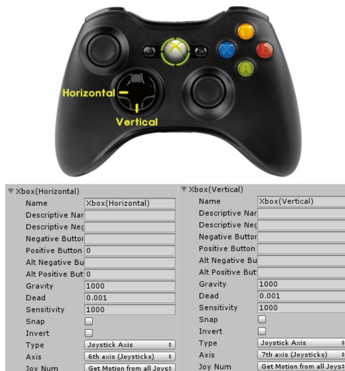
Figure 7. Key setting process of the game pad controller.
