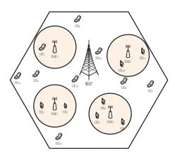
Figure 1. Macro-cell access point-femtocell access points (MAP-FAPs) heterogeneous network model.
