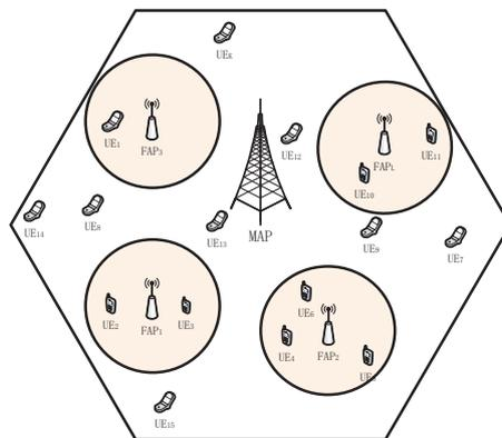
**Figure 1.** Macro-cell access point–femtocell access points (MAP–FAPs) heterogeneous network model.
