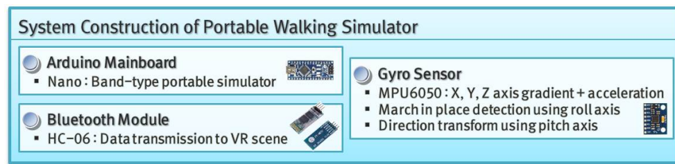
Figure 5. System components and roles of the portable walking simulator.
