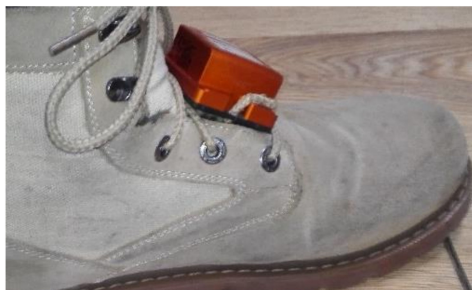
Figure 3. The IMU tied on the left foot.
