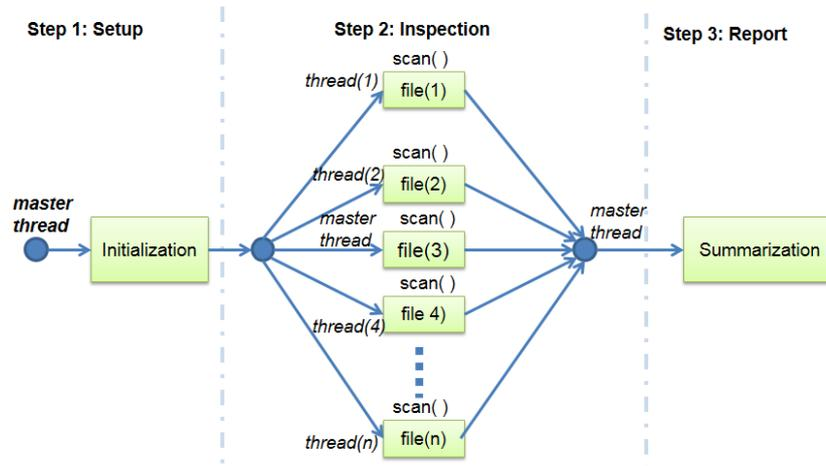
Figure 3. ClamAV's parallel diagram processing (single file per thread).
