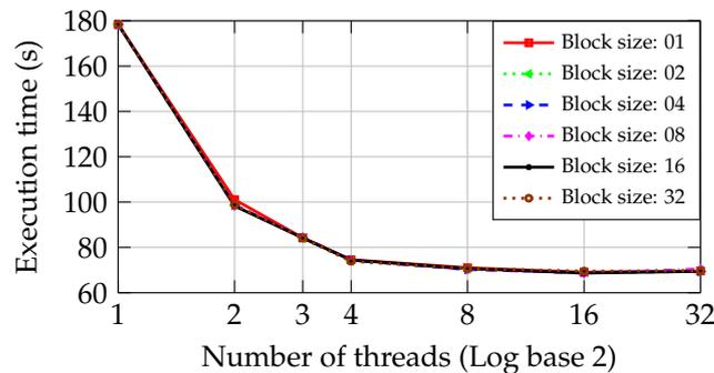
Figure 11. Execution time in the guided approach in the PC with I5 CPU.
