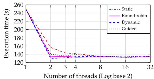
Figure 14. Comparing the four approaches in the PC with Core2 CPU.
