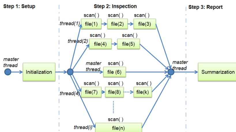
Figure 4. ClamAV's parallel diagram processing (multiple file per thread).
