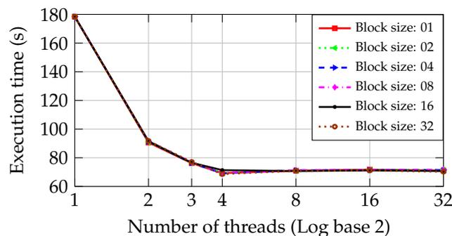
**Figure 9.** Execution time in the dynamic approach in the PC with I5 CPU.
