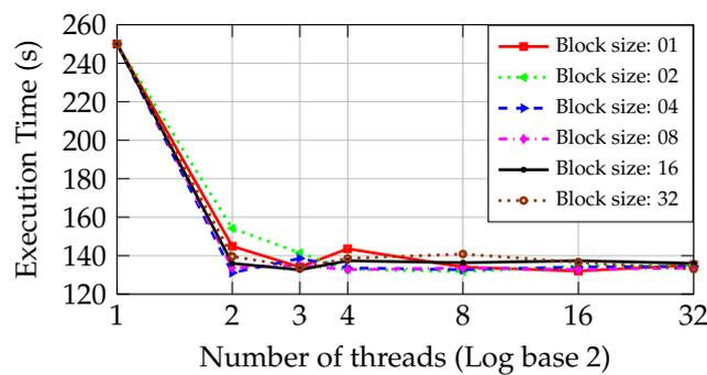
**Figure 8.** Execution time in the round-robin approach in the PC with Core2 CPU.
