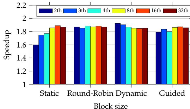
Figure 22. Speedup comparing the four approaches in the PC with Core2 CPU.
