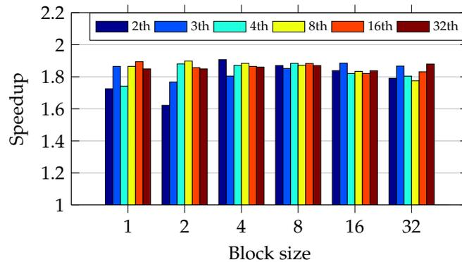
**Figure 16.** Speedup with the round-robin approach in the PC with Core2 CPU.
