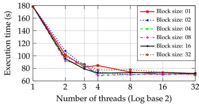
**Figure 7.** Execution time in the round-robin approach in the personal computer (PC) with I5 central processor unit (CPU).
