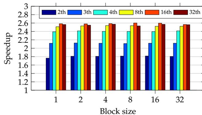
**Figure 19.** Speedup with the guided approach in the PC with I5 CPU.
