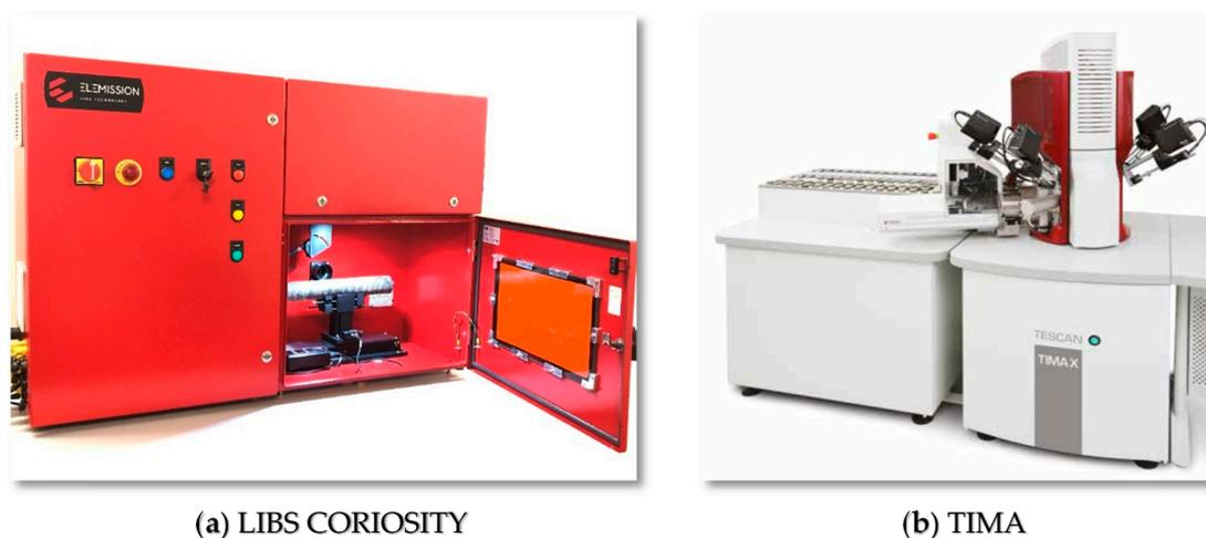
**Figure 1.** (a) LIBS CORIOSITY mineral analyzer and (b) TIMA-X with a 100-sample autoloader.
