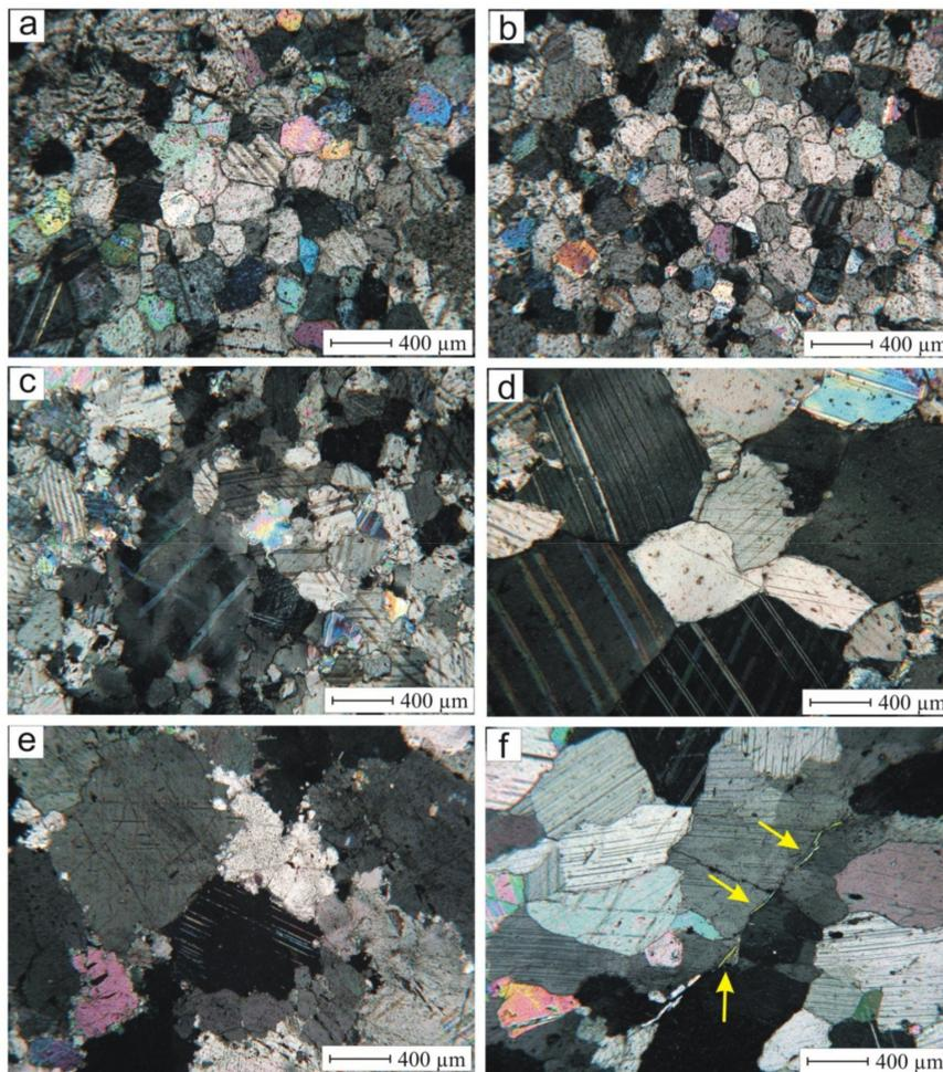
**Figure 3.** Microphotos in thin section by polarized optical microscopy, images under crossed nicols. (a) Sample C2; (b) Sample C11; (c) Sample C13; (d) Sample C14; (e) Sample C18; (f) Sample C20, where microcrystals of white mica are visible.
