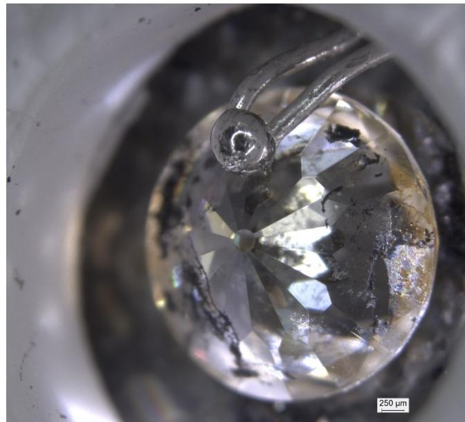
**Figure S1.** Pt-Pt/Rh thermocouple, touching the surface of the diamond.
