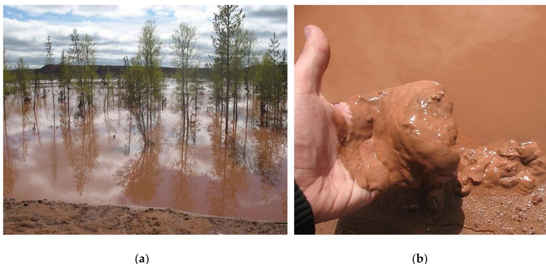
**Figure 2.** Kimberlite processing waste: (a) the settling pond and solids of the beachside terrain; (b) close-up view of the characteristic slurry with the predominant (85%) particle size class of  $<25\ \mu\text{m}$  [54].
