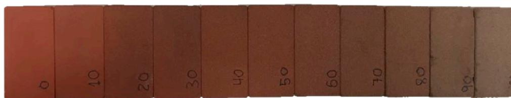
**Figure 6.** Image of the samples of the different families of ceramics conformed from clay and mining waste. From left to right, 0M10C, 1M9C, 2M8C, 3M7C, 4M6C, 5M5C, 6M4C, 7M3C, 8M2C, 9M1C and 10M0C.
