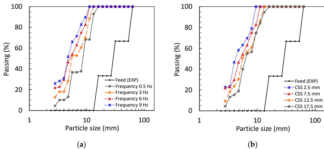
**Figure 15.** Product particle size distributions for different stroke frequencies and a constant CSS of 7.5 mm (a) and for different closed side settings for a fixed frequency of 6 Hz (b) in DEM simulations of the laboratory jaw crusher for a feed particle size distribution (Table 5).
