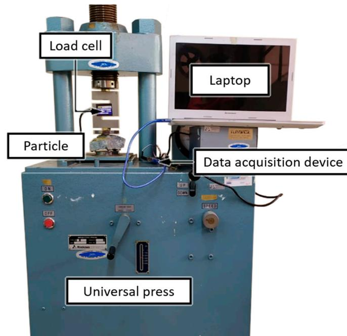
**Figure 4.** Uniaxial compression system used in unconfined testing of particles.
