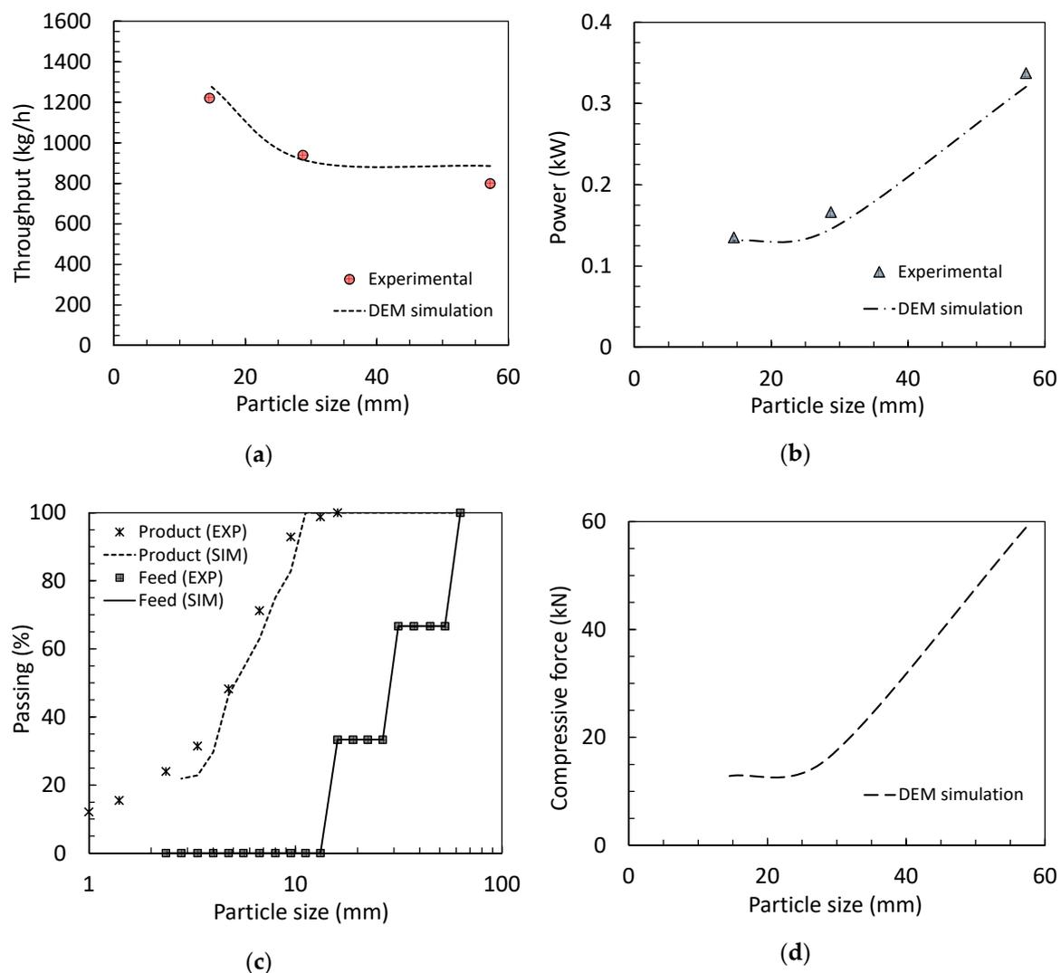
**Figure 14.** Comparison between experiments and DEM simulations for the jaw crusher throughput (a), power (b) and product size distribution (c); simulated trend on the compressive force (d). Figures a, b and d presented as a function of mean feed particle size.
