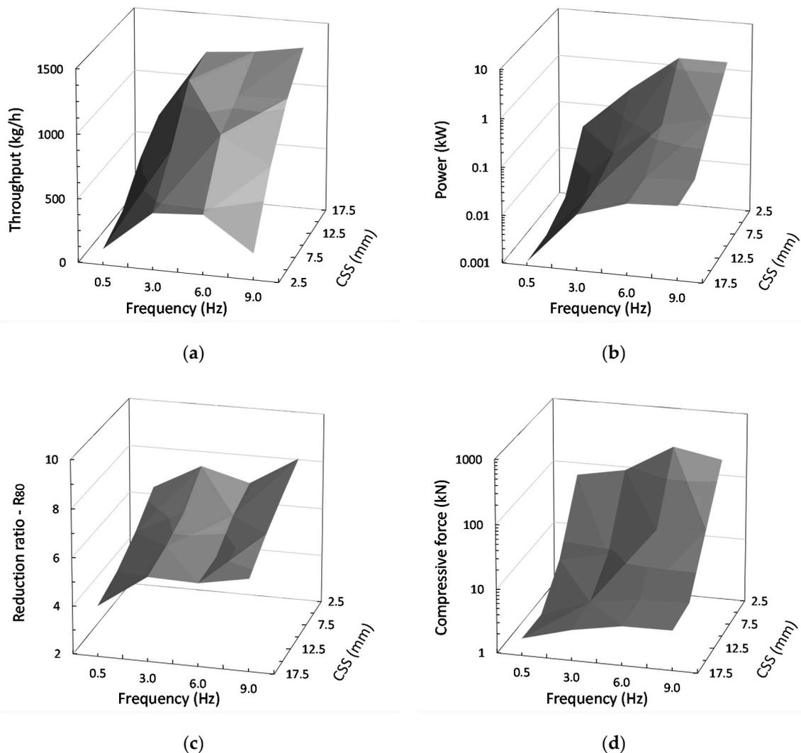
**Figure 17.** Response surface analysis of the jaw crusher DEM simulations showing throughput (a), power (b), reduction ratio (c) and compressive force (d) as a function of closed side setting (CSS) and stroke frequency.
