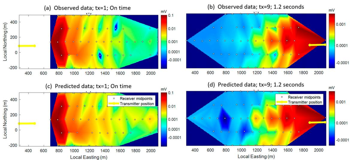
**Figure 12.** Maps of predicted (top panels) and observed (bottom panels) data. The columns of images show the results for different transmitter positions. The left column is transmitter one (indicated by the yellow line) during the on-time and the right column shows data for transmitter #9 at 1.2 s.
