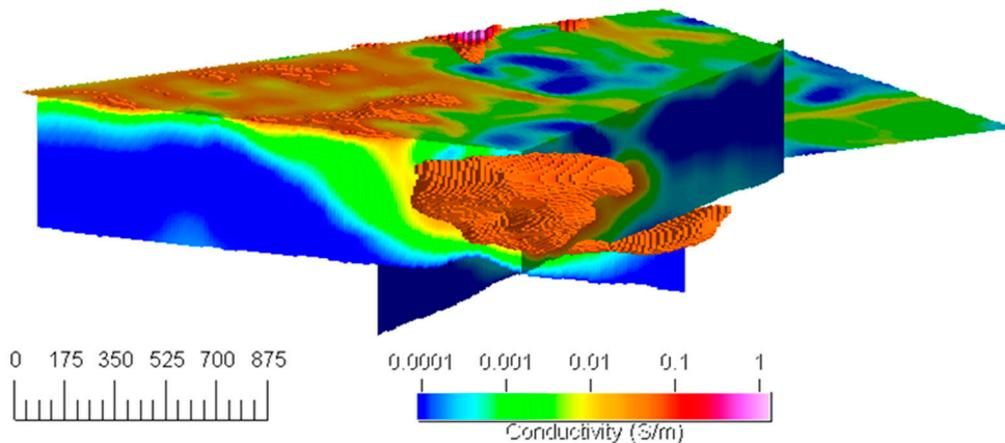
**Figure 3.** Conductivity volume of prospective target from the results of the airborne survey inversion. The cut-off shows conductivity greater than 0.05 S/m. The conductive overburden is shown in the near surface. The color map is conductivity in S/m, and the scale on the left shows distance in meters.
