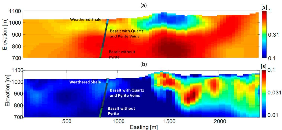
**Figure 16.** Inversion results of the times constant under the center line of the 3D array, along the profile shown in Figure 4. The top panel (a) shows the results from the distributed array, and the bottom panel (b) shows the results from the 2D dipole–dipole lines.
