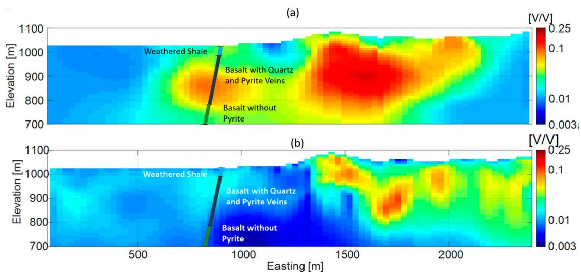
**Figure 15.** Inversion results of the chargeability under the center line of the 3D array, along the profile shown in Figure 4. The top panel (a) shows the results from the distributed array, and the bottom panel (b) shows the results from the 2D dipole–dipole lines. The position of the borehole and preliminary qualitative estimates of the types of the rocks from the drilling are overlaid on the images.
