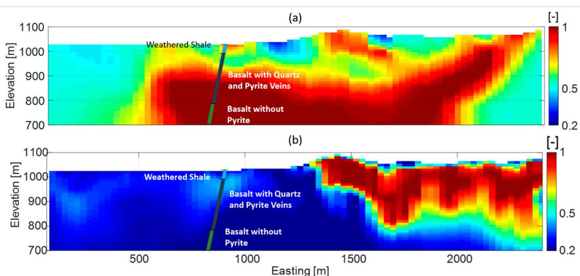
**Figure 17.** Inversion results of the relaxation coefficient under the center line of the 3D array, along the profile shown in Figure 4. The top panel (a) shows the results from the distributed array, and the bottom panel (b) shows the results from the 2D dipole–dipole lines.
