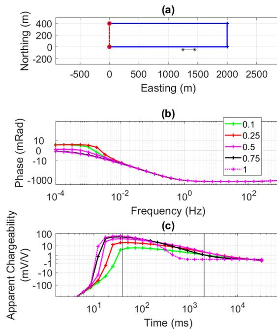
**Figure 10.** Relaxation constant distinguishability for 3D configuration with the transmitter wire near the receiver wire and a 100 Ohm-m half space. Panel (a) shows the source-receiver layout. Panel (b) shows the frequency domain phase. Panel (c) shows the time-domain apparent chargeability. The color of the plots corresponds to a relaxation constant of the medium—from 0.1 (bold green line) to 1 (dotted pink line). The two vertical lines in panel (c) show the time range of the current system.
