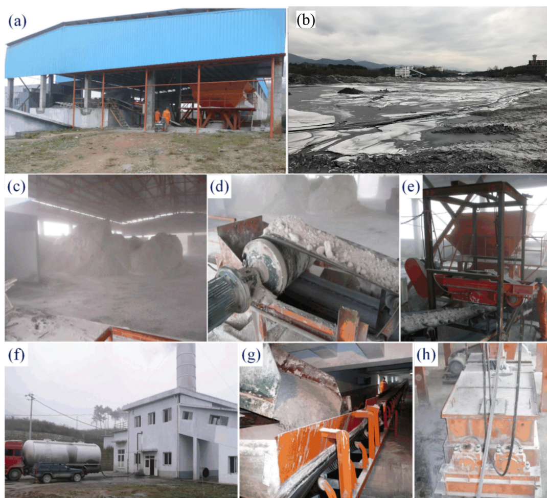
Figure 6. (Source: Kai-lin Group Co., LTD, Guiyang, China) Configuration diagram of the Kai-lin Mine Backfill system in the mining industry: (a) panorama of backfill station; (b) phosphogypsum storage yard (outside); (c) phosphogypsum storage yard (inside); (d) phosphogypsum conveyor; (e) stable hopper; (f) cement silos; (g) belt conveyors; and (h) horizontal double-shaft mixer.
