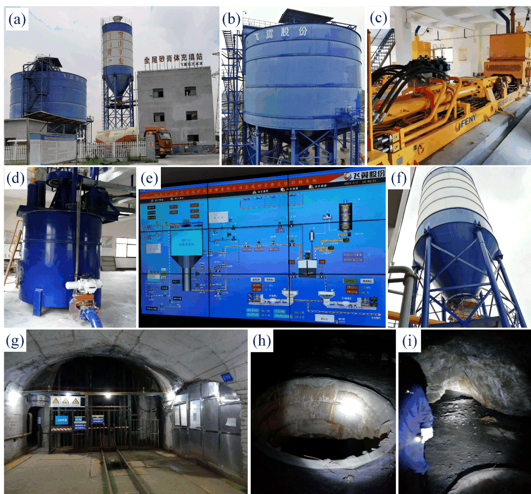
Figure 7. (Source: Hunan Baoshan Mining Co., LTD, Chenzhou, China) Configuration diagram of paste backfill system of Hunan Baoshan Mining Co., LTD: (a) panorama of backfill station; (b) deep cone thickener; (c) backfill industrial pump; (d) vertical stirring drum; (e) control systems; (f) cement silos; (g) man-material shaft; (h) stope chute; and (i) backfill body exposed in stope.
