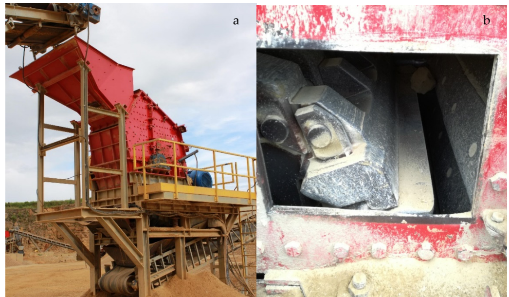
Figure 2. Crushing device—impact crusher KU 65-120 during investigations (a); calibrating gap in the crusher (b).
